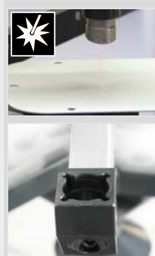
Laser pointer for optical display of tool centre and power bank
