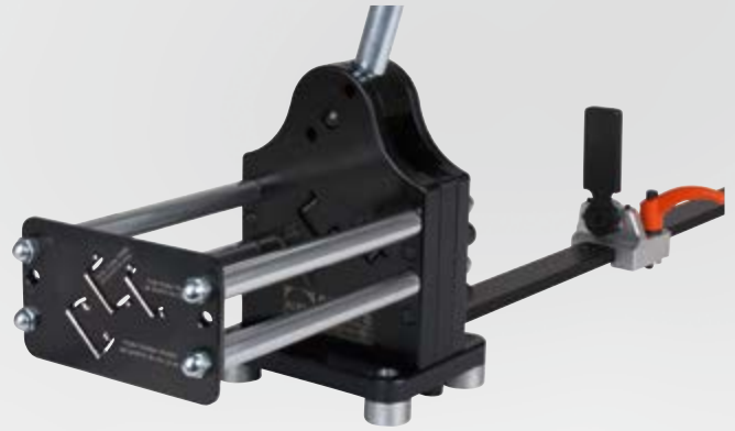
Guidance fixture for 90° angle-precise cutting
