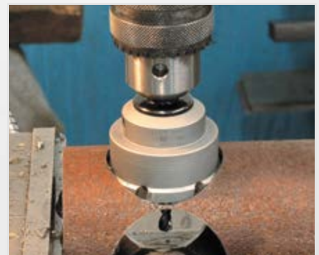
Drilling in pipes
