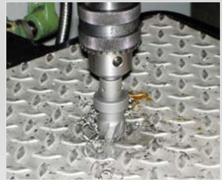
Drilling structured sheet metals
