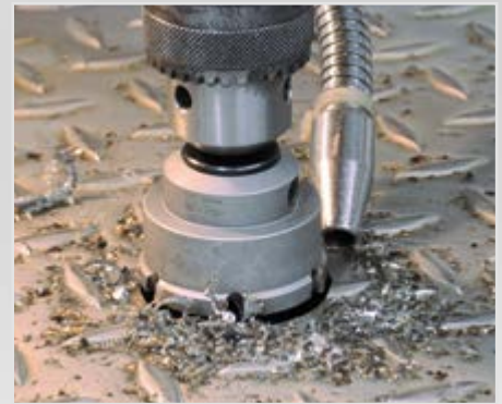
Drilling in checker sheet
