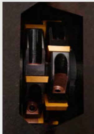
2 milling disks together with 6 inserts each
