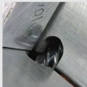
Precise deburring by rolling milling
