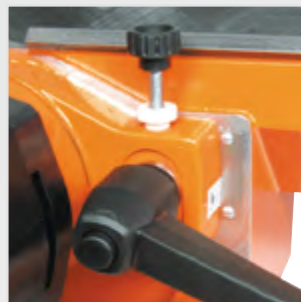
Fine adjustment to milling depth/bevel width
