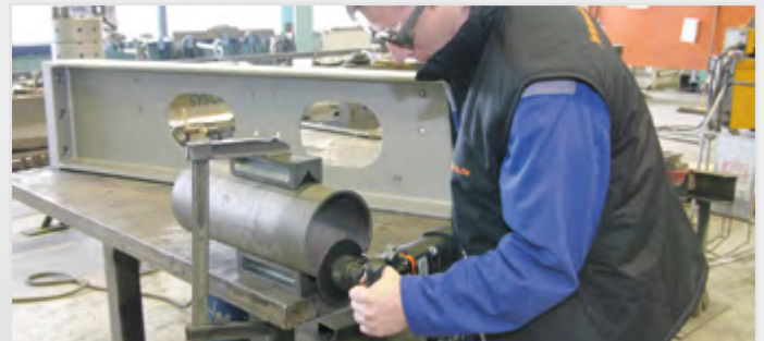
Start holes from \varnothing 20 mm.
