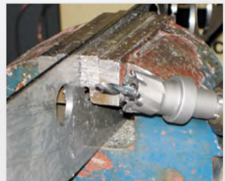
Free-hand drilling up to Ø 30 mm
