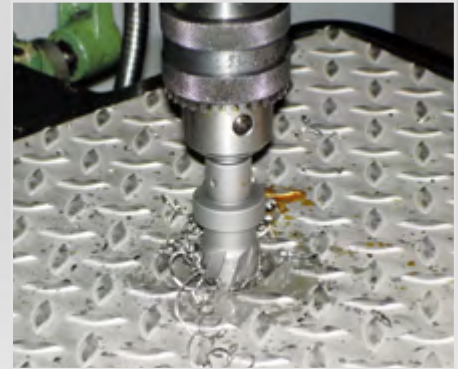
Drilling structured sheet metals
