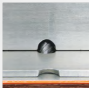
Position II: Material thickness from 1.5 mm
