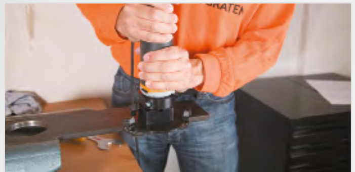
Initial drill holes from: \varnothing 3.0 mm for pin cutters \varnothing 5.0 mm in spherical cutters
