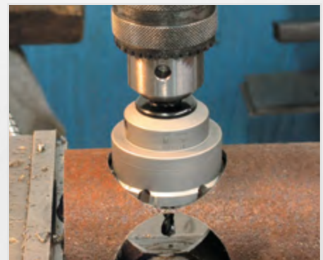
Drilling in pipes
