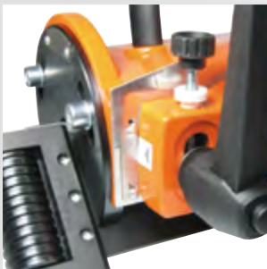
Fine adjustment to milling depth/bevel width
