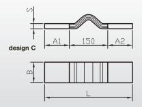
The expansion connectors in the following tables consist out of copper HCP-foils according to DIN EN 13599 with a thickness of 0,1 mm or 0,3 mm. The contact areas are manufactured in a press-welded design.
