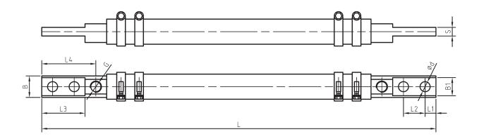
Water cooled hollow core cables 300-1000 mm<sup>2</sup> for medium frequency up to 2000 hertz
