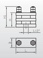
Insulators in doubled hexagonal design with threaded steel inserts (9S 20 K zinc coated)
