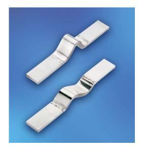
The laminates of our standard aluminium expansion connectors consist out of pure aluminium foils with a thick-ness of 0,3 mm. As contact areas we use solid aluminium pieces. They are welded by an electrical arc and shielded with inert gas to prevent oxidation of the molten bath.
