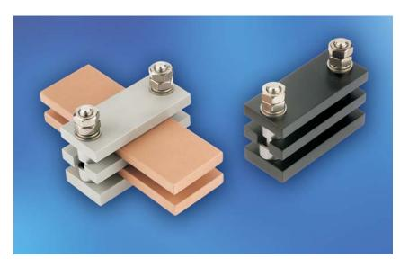
Busbar supports for use as **sliding** support for long busbars which must slide in the holder to allow the thermal expansion. By using this design the lower part of the holder is fastened to the support by means of the stay bolts prior to assembly. Now a simple insertion of the busbars between the stay bolts is possible and a time saving assembly is realized.
