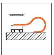
Connections between fixed machine parts and movable switching devices
