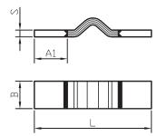
Flexible transformer connections with expansion part
