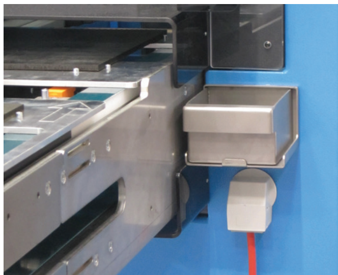
KVT 50-W90 Low profile 90 degree routing of a terminated cable from a control panel into the machine
